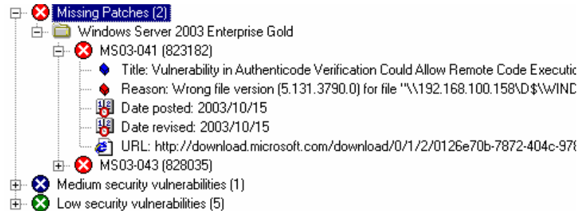
Missing patch sample output in scan results tree
